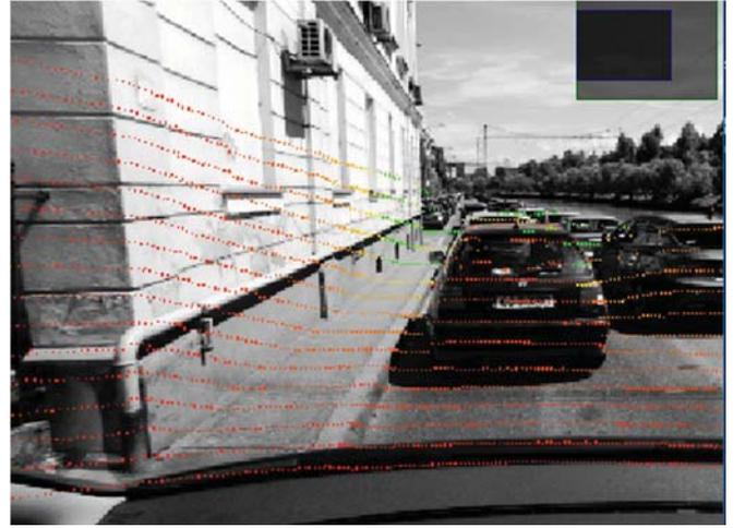
Figure 5. Projection of LIDAR points on grayscale image obtained from the camera
