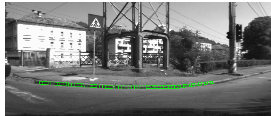
Fig. 12. Better results are obtained using vertical alignment of each curb segment.
