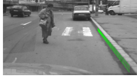
Fig. 10. The curb segment projected back onto the left image, for the scene shown in figure 2.
