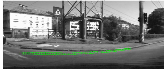
Fig. 11. The chain of curb segments projected back onto the left image (the vertical coordinate of curb points is the road level from calibration), for the scene analyzed in figure 9.
