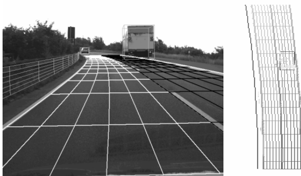
Fig. 13. Guard rail and side lane detected on highway
