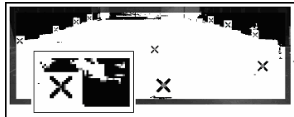
Fig. 2. Concavities detection: zoomed area – upper/lower/ left/right concavities; complete image – centers of detected groups of 4-concavities are marked.
