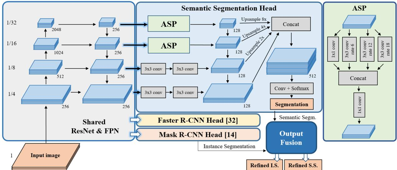
Fig. 1: A shared ResNet-FPN network is used for 3 tasks. The Faster-RCNN head performs object detection, Mask-RCNN head performs instance segmentation. Our semantic segmentation head is based on Atrous Spatial Pyramid (ASP)
