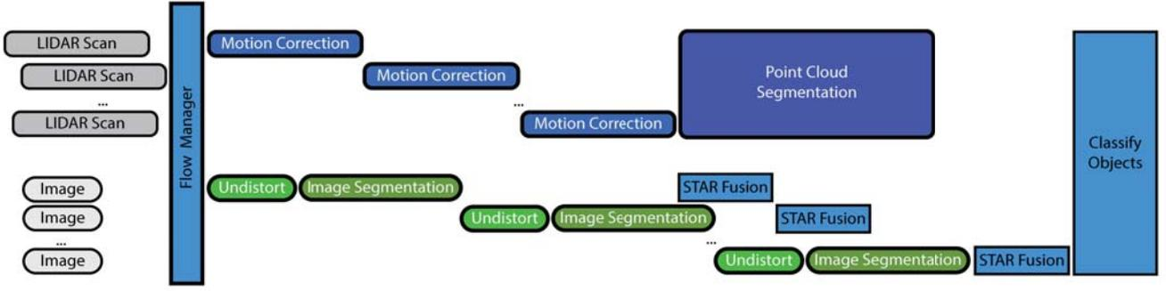
Fig. 2. Typical timeline of an execution cycle of the processing chain (time progresses left to right)
