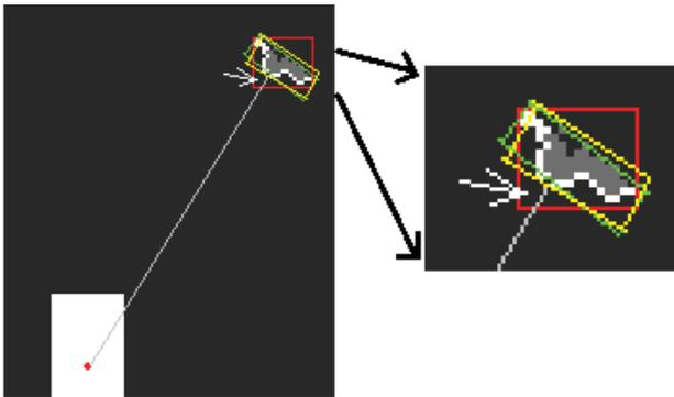
Fig. 9. When the dominant line  $L$  is less reliable, the line of sight can be used to infer the obstacle orientation, as the yellow cuboid. The un-oriented cuboid is shown with red, and the cuboid given by  $L$  with green. The line of sight to the obstacle center is shown. The white arrow depicts the free area, visible to the perception system, which is computed for each cuboid.
