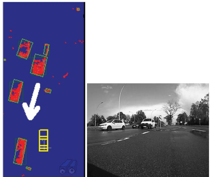
Fig. 10. Scenario 1 used for evaluation. Incoming traffic (the direction of motion shown with the white arrow) at an angle of 14.4 degrees.
