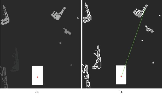
Fig. 3. a. Scenario from Fig. 1 with different labels for each obstacle, the ego vehicle is the white rectangle and the red dot represents the reference point for the perception system, b. Each obstacle patch has its boundary cells marked (white points), and an example of line of sight from the perception system to a boundary cell is shown as the green line.
