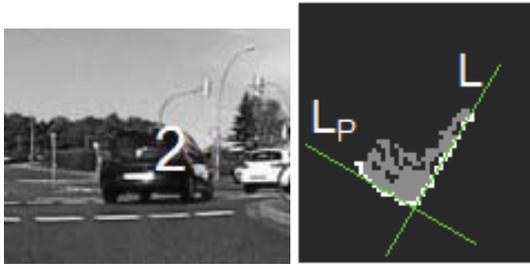
Fig. 5. The two lines computed for the vehicle 2 are shown (the scenario presented in Fig. 1).
