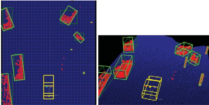
Fig. 6. The oriented cuboids for the scenario presented in Fig. 1 are shown with bright green, in top-view (left) and a perspective view of the scene (on the right).
