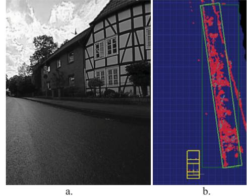
Fig. 7. a. Scene with a large fence + building on the right side of the road, b. Top-view of the oriented (bright green) and un-oriented obstacle (dark green) detected from the 3D data of the fence and nearby vegetation.
