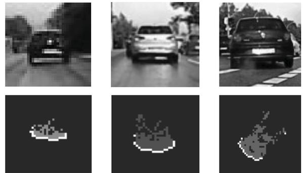
Fig. 8. Small passenger cars that are viewed from the rear (or front), without perceiving one of the lateral sides, often present curved visible boundaries that are less reliable to fit lines.
