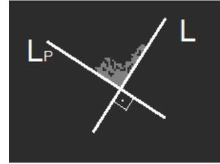
Fig. 2. The two lines used to model oriented objects: L will be fitted to the dominant visible side (the longest visible side of the obstacle), while  $L_P$  will model the other visible side, if any.
