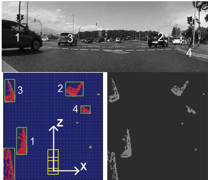
Fig. 1. Input of the proposed approach: a set of detected obstacles, with un-oriented cuboids (green). Top image: a camera view in front of the ego vehicle (yellow in the top view), with four relevant obstacles marked, 1,2,3 - vehicles, 4 - bicyclist. Bottom-left: the result of obstacle detection (red areas), a bird-eye view, bottom-right: occupied grid cells are shown with a medium grey shade.
