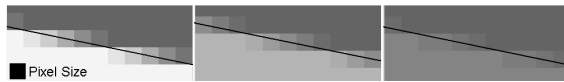
Fig. 6. Samples of strong, normal and weak edges are shown together with the true edge line (black) with the slope 0.2.
