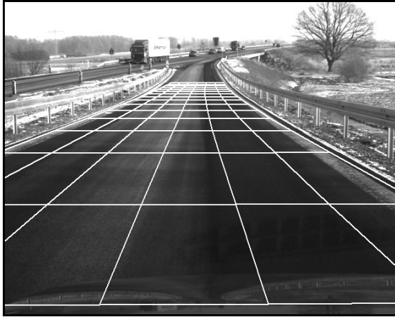
Fig. 6. Results of lane detection on non-flat roads with vertical curvature.
