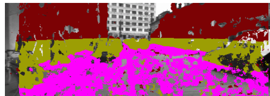
Fig. 4. Road points, relevant points for obstacle detection and irrelevant high points
