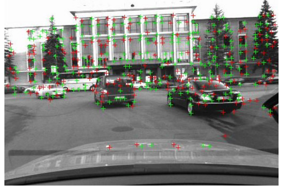
Figure 2 Features marked in red are rejected by the two way optical flow
