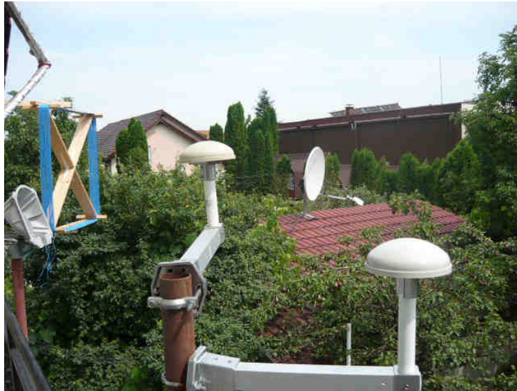
Fig. 4. The antennas of the two GPS receivers, placed on the same pole.
