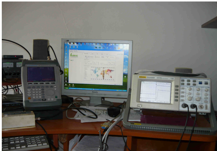
Fig. 5. The equipment used for measuring the time delay.
